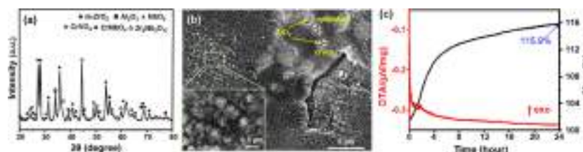
Fig. 2. Result of 24 hours high-temperature oxidation behavior at 900 °C (a) XRD result of RHEA, (b) SEM-SE image of RHEA (c) TG-DTA curve
